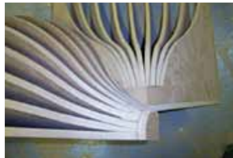
制作胶合板模具 Plywood male and female mould
