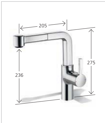
Lever mixer lever installation possible on the right or left side pull-out spray with KWC JETCLEAN hose guide, swivelling 360°
